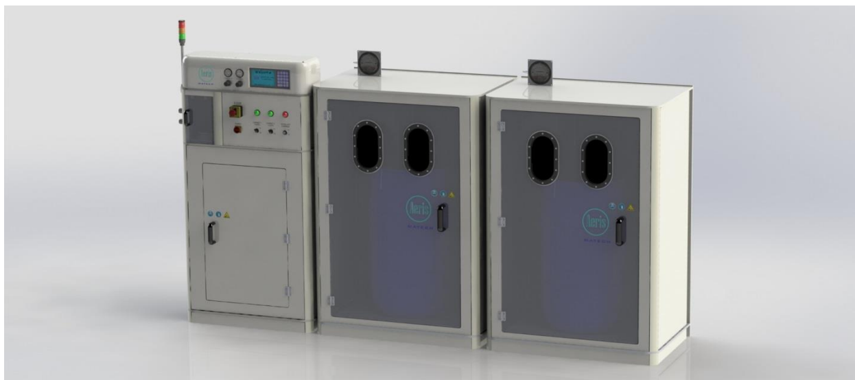
Figure 3. Aeris™ Precision system configured with two 55 gal drum delivery cabinets. On the left is the control console, on the right, the two drum cabinets. Carboy and bottle cabinets are also available and can be configured in any combination.
